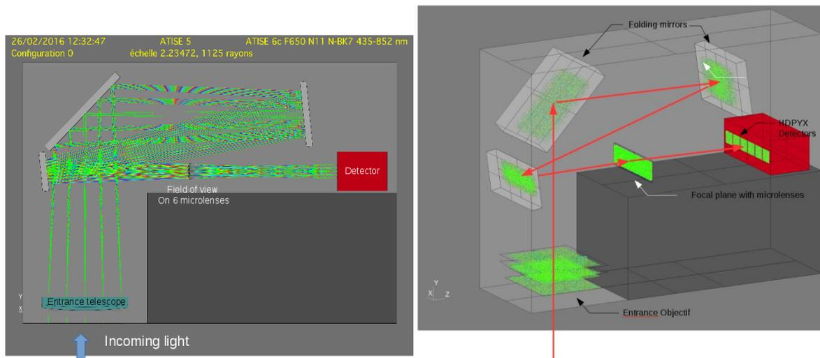
**Fig. 4.** a) ATISE optical schematic. b) Perspective view showing light distribution on each optical surface. The optics forms an image of entrance pupil on detector which create an uniform illumination corresponding to one of six line of sight.
