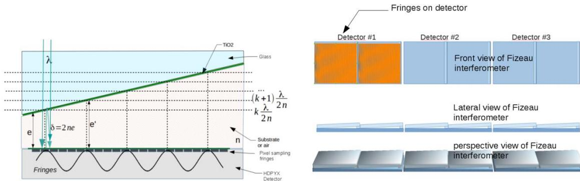
**Fig. 5. a)** SPOC principle : A semi-transparent plate is set on top of detector. Light coming from observed field of view reflects both on semi-transparent plate and detector itself. Fringe pattern formed by interference is measured by detector. Fourier transforms of this image gives the spectra corresponding to whole field of view concern by this way. **b)** An HDPYX detector is divided in two zone with one interferometer by zone. 3 detectors permits us to select 6 lines of sight
