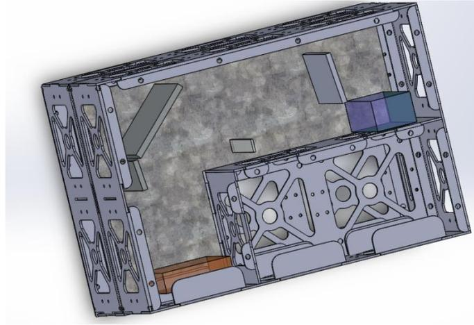
**Fig. 3.** ATISE Mechanical implementation for optical test assembled with 6U platform.
