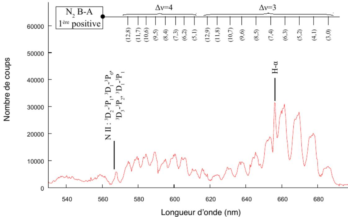
**Fig. 1.** Spectrum of the auroral simulator planeterrella (ref papier Jean) between 520 and 700 nm. The resolution is around 1 nm. The spectrum of the aurora is somehow different since forbidden transitions also appear in aurora and airglow mainly O<sup>1</sup>S at 557 nm and O<sup>1</sup>D triplet at 630, 639 and 639 nm
