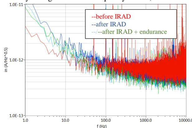
Fig. 11. Current noise spectral density before and after irradiation and endurance at a reverse bias of 12 V.
