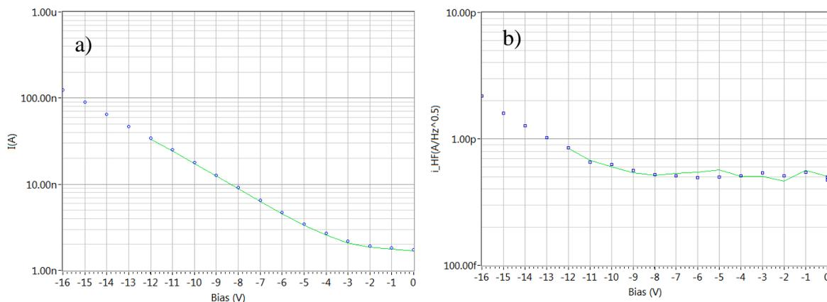
**Fig. 10.** Variation of a) output current and b) average current noise spectral density as a function of reverse bias before (continuous line) and after (squares) proton irradiation.
