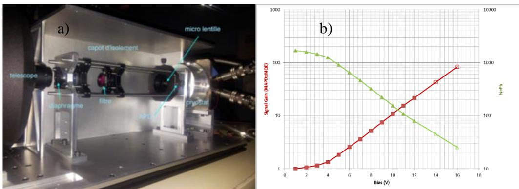
**Fig. 6.** a) Integration of the MCT APD detector module in the COWI LIDAR set-up and b) measured APD gain and sensitivity of 200 μm MCT APDs detector modules operated at 190 K with a bandwidth of 14.5 MHz
