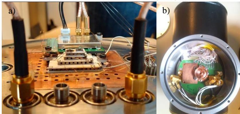
**Fig. 5.** Images of a) the high temperature TEC cooled detector module and b) the LN2 cryostat.
