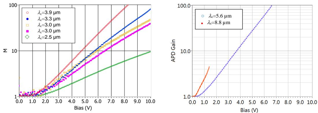
Fig. 2. MCT APD gain measured at  $T=80$  K for APDs with cut off wavelengths ranging from 2.5 to 8.8  $\mu\text{m}$ .
