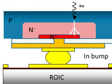
**Fig. 1.** Illustration of a backside illuminated planar HgCdTe APD made at CEA/Leti.
