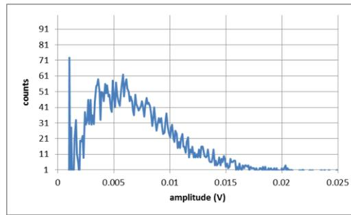
**Fig. 3.** Estimation of the APD gain PDF from asynchronous detection of thermal single photons and by subtracting ROIC noise and dark current events. The corresponding excess noise factor is equal to  $F=1.23$
