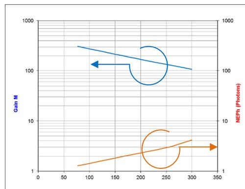
**Fig. 8.** Modelled APD gain and sensitivity (NEPh) of 15  $\mu\text{m}$  with  $\lambda_c=2.8 \mu\text{m}$  HgCdTe APD operated at fixed bias (17.5 V) and coupled with a 10 GHz bandwidth TIA with an equivalent input current noise density of 10  $\text{pA}/\sqrt{\text{Hz}}$ .
