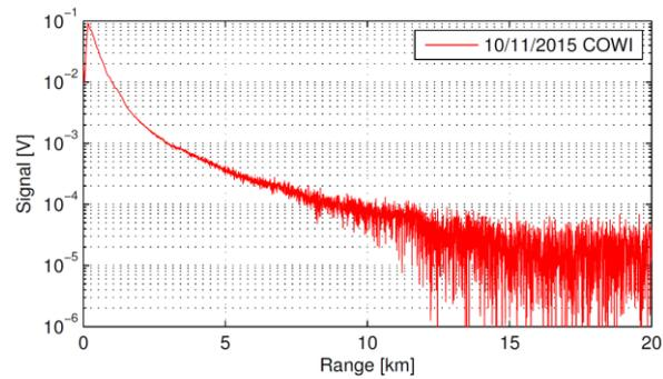
**Fig. 7.** Return signal collected with MCT APD in the COWI set-up with an. The return signal from a distance corresponds to about 1 photons per 25 ns (BW=20 MHz)
