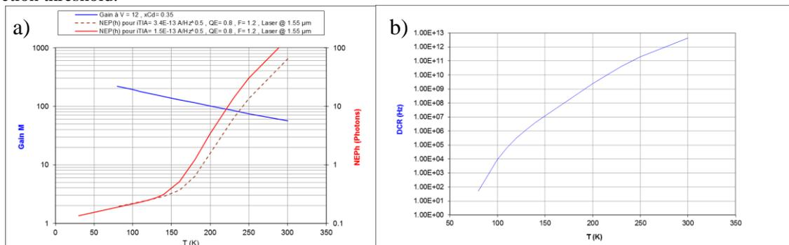
**Fig. 9.** a) Modelled sensitivity of MCT APD detectors with a diameter of 30  $\mu\text{m}$  and  $\lambda_c=3.6 \mu\text{m}$  coupled to low noise pre-amplifiers with a noise of 33 electrons rms over 0.2 and 1 GHz and b) associated DCR.
