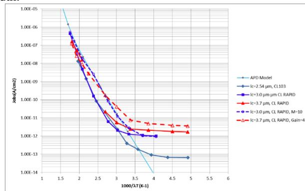
**Fig. 4.** Gain normalised dark current compared to modelled dark current as a function of the  $\lambda_c$  normalised inverse temperature for APDs with an without gain and with  $\lambda_c$  varying from 2.5 to 3.6  $\mu\text{m}$
