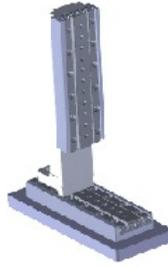
Figure 3. 3D view of the bi-axis system with the smaract piezo-positioners
