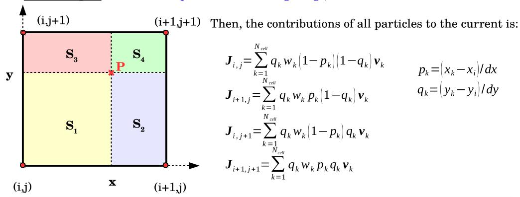
Even though the particles are point-like, they have an **effective size** that is felt through the deposition of currents on the grid. In this case, their effective shape is triangular.
