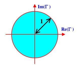
The domain of definition of the reflection coefficient is a circle of radius 1 in the complex plane. This is also the domain of the Smith chart.
