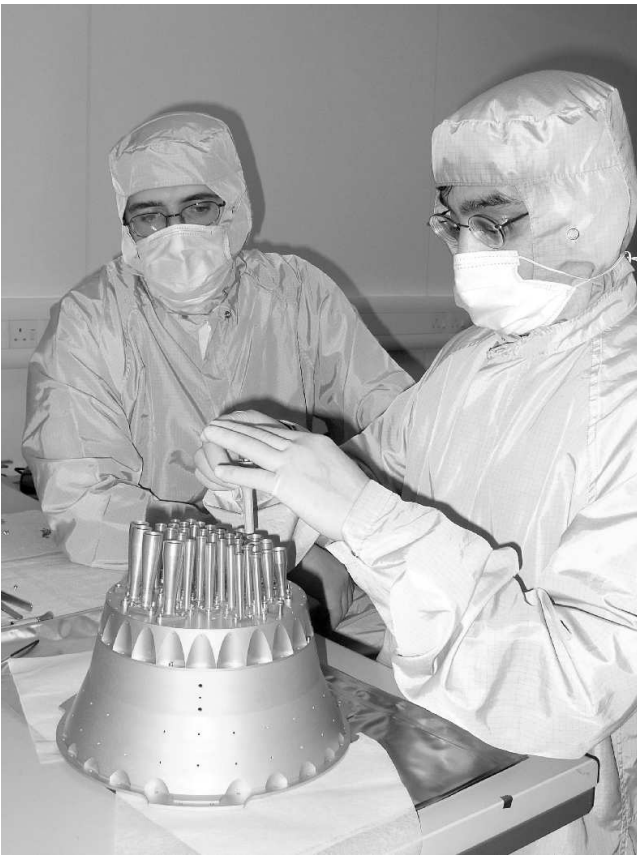
Figure 4. Integration of the 4 K HFI Back-to-Back horns. Each horn couples the telescope to one detector assembly. Note the curvature of the focal plane (top of the back-to-back horns) due to the chosen off-axis Gregorian PLANCK telescope.
